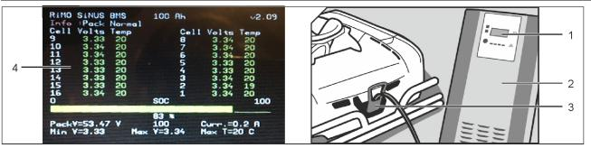
Fig. 47: BMS LCD display and charger
