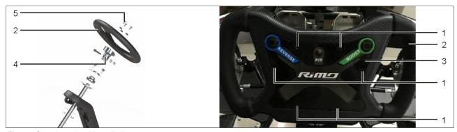
Fig. 41: Steering wheel installation
