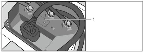
Fig. 24: ACD motor controller
